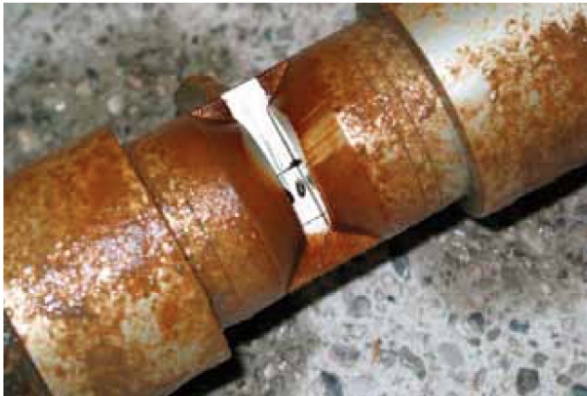
Figure 9: Efficiency of the automatic cleaning - the sensor is dirty but the measuring path is free of fouling
